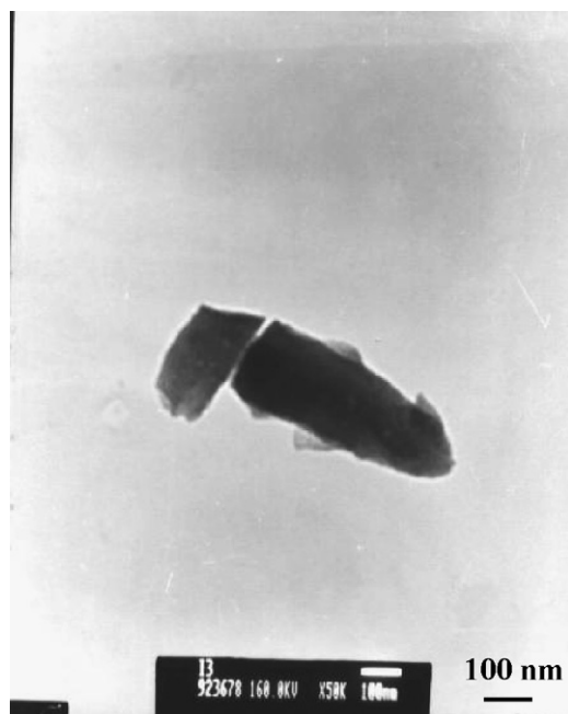
Fig. 8. TEM image of sample E ( \text{Fe}(\text{OAc})_2 and \text{IPA}/\text{H}_2\text{O} ) with rectangular morphology.
